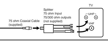
NOTE: If a VHF or UHF antenna is used, set the TV/CATV menu option to the "TV" mode.
